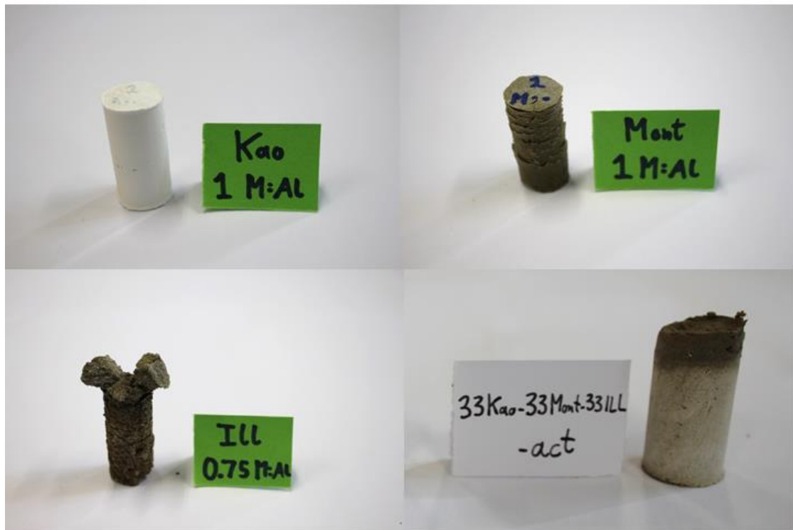
Figure 4: Photos of activated samples of kaolinite, montmorillonite, illite, and a mixture of all three.
