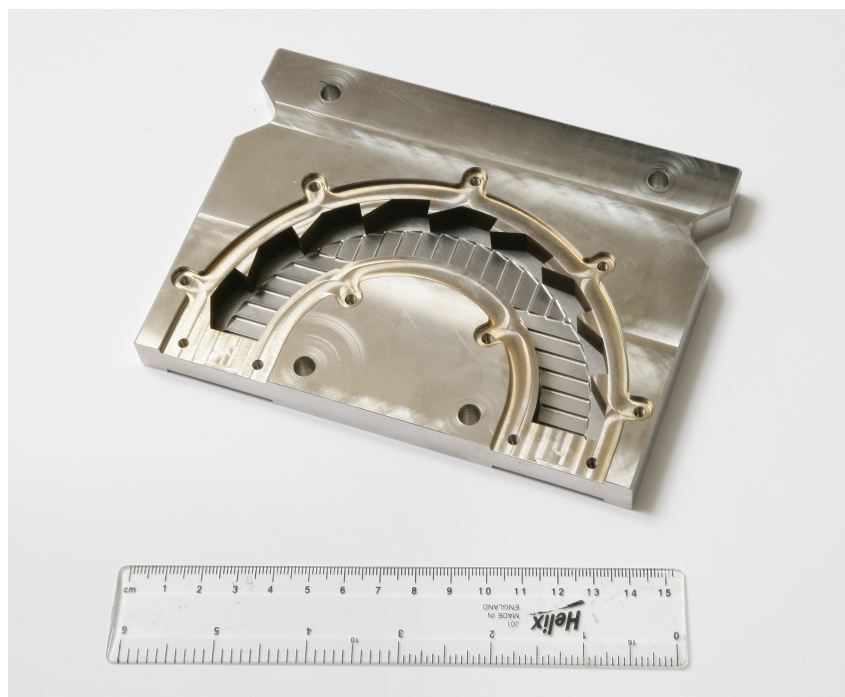
Figure 4.20: Image showing the interior of the flight tube that is placed into the air gap of the magnet during assembly. After the magnet is placed over the chamber, ions that enter the circular arc will be deflected by the magnetic field and ions with a specific m/z ratio will make it around the semicircular path without colliding with the chamber wall. The serrated edges prevent ions that collide with the chamber wall from reaching the exit of the magnetic sector. Photograph taken by workshop technician Kevin Mott
