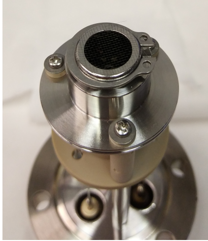
Figure 4.36: Image of the top of the electron multiplier with a grid over the entrance to shield the multiplier from external fields. The grid is held in place by a circlip over the entrance of the multiplier.
