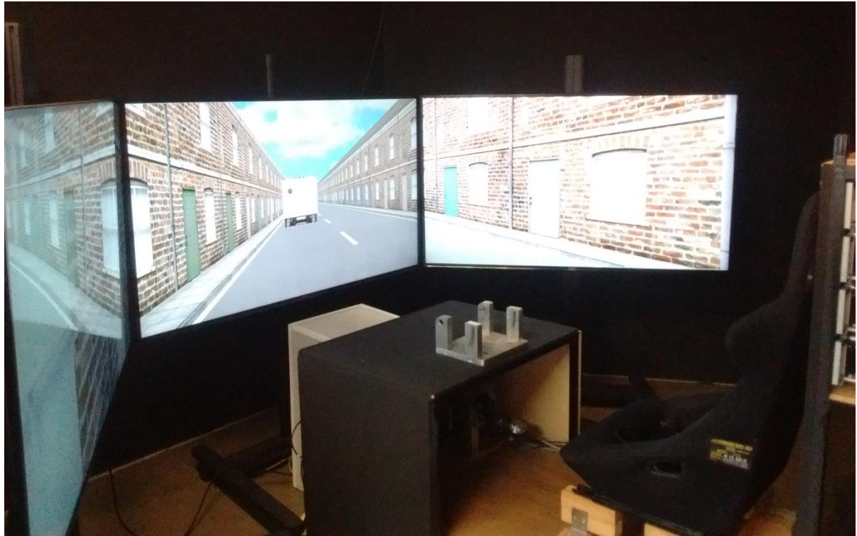
Figure 3-19 – Driving simulator set up for a car following scenario
