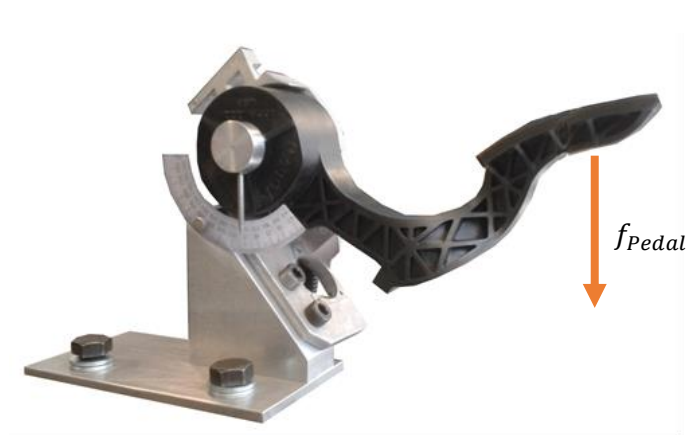
Figure 3-6 – Volvo accelerator pedal measurement rig
