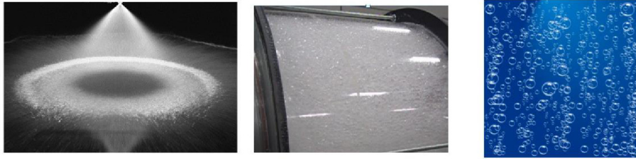
Figure 6.1: Comparison of three methods for creating large contact area between a liquid and gas: spraying, foaming and bubbling [5]
