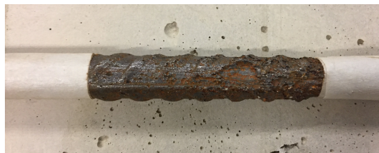
Figure 15: Spalling of corroded steel on specimen A10-15a
