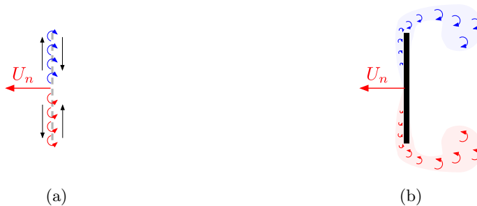
FIGURE 2. Schematic comparing vorticity distributions between potential flow (a) and a viscous flow field (b). In the viscous fluid vorticity is diffused and advected from the plate surface, whereas vorticity is contained in an infinitely thin layer for the inviscid fluid. Red and blue colours correspond with positive and negative vorticity respectively.
