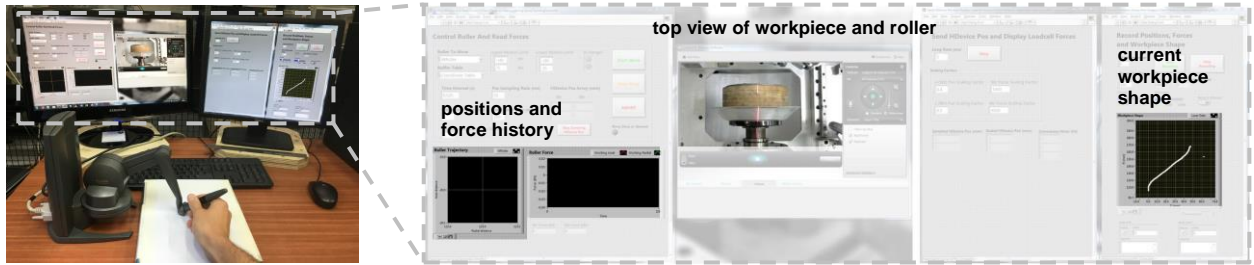
Fig. 3. The haptic spinning desk set-up. The operator holds the haptic device stylus like a pen over a wide flat support. On the computer screens, a webcam and several charts provide the operator with visual feedback on the progress of forming: positions, forces and workpiece shape.
