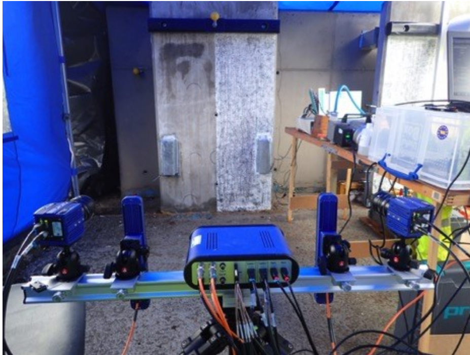
316 317 Figure 10 Digital Image Correlation camera and tripod set-up on the microcapsule wall.
