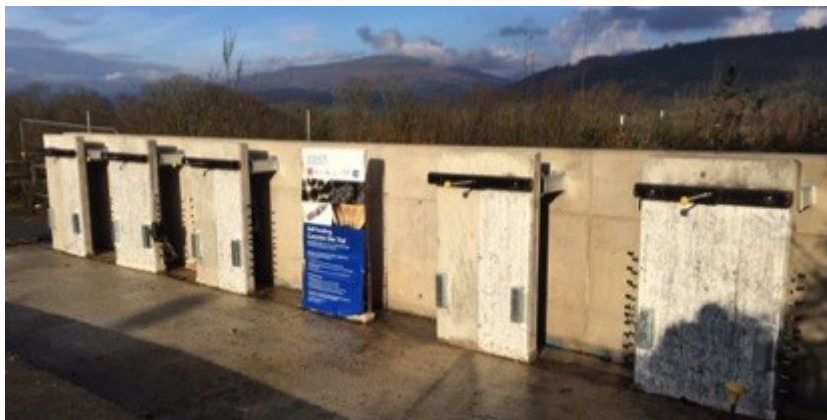
215 216 Figure 3 Self-healing concrete wall panels constructed within the EPSRC and industry funded 217 Materials for Life (M4L) project [35].
