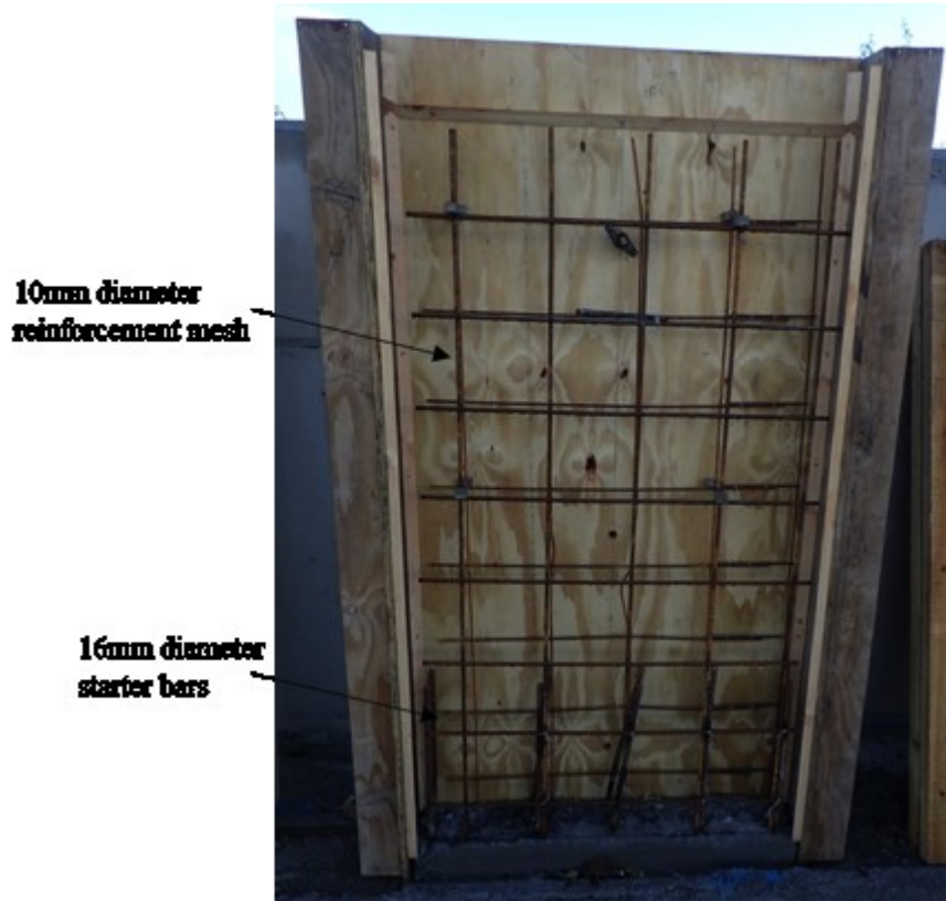
271 272 Figure 5 Wall panel reinforcement design to ensure cracking at ~500mm from the base of the wall 273 panel.
