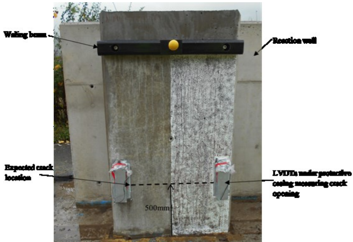
274 275 Figure 6 The microcapsule wall panel half painted with a black-and-white speckle pattern for DIC 276 analysis
