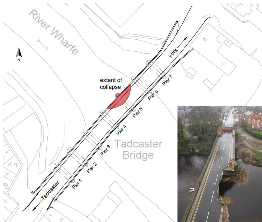
Fig. 1. Bridge schematic showing location of bridge and extent of collapse. Photo of collapse site taken after flooding receded. Imagery provided courtesy of North Yorkshire County Council and annotated by authors.
