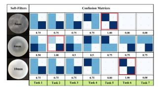
Fig. 8: Confusion matrices and accuracy values for 7 different tasks corresponding to the clustering results obtained with three soft filters of 3mm, 6mm and 10mm respectively. The diagonal in each matrix retains the counts for the correct cluster guesses. Each soft filter is optimized for a specific task, highlighted in red.
