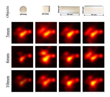
Fig. 6: 3D-printed Sphere, Cube, Half-Cylinder and Cuboid (view from above) and relative tactile images computed (averaged sensor readings over three trials).
