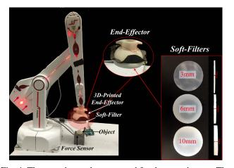
Fig. 4: The experimental set-up used for the experiments. The ST robot was used to push the sensorised end-effector against the object. A FlexiForce sensor A502 from TekScan was used for controlling the normal force applied. Three different soft filters were used in the experiments
