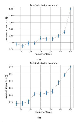
Fig. 10: The figure reports the average accuracy and error  $e = \pm \frac{\sqrt{std}}{N}$  for the inference algorithm to cluster according to Task 4 (a) and Task 5 (b), when morphologically processing the data with their respective optimal filters (3mm soft filter and 10mm soft-filter respectively).
