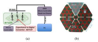
Fig. 3: (a) The CySkin technology architecture. The hexagonal patch is connected to a Intelligent Hub Board (IHB) that collect the tactile sensor data and send them to the PC through a CAN bus. (b) The CySkin patch used for the experiments. It is composed by 6 interconnected triangular modules, each hosting 10 taxels.
