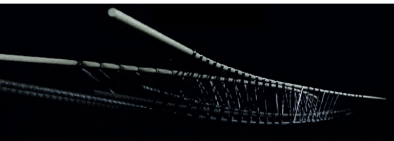
Fig. 3: FRP optimized reinforcement cage
