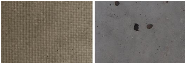
Figure 6: Fabric cast (left) and Timber cast surface (right), from the same concrete mix.
