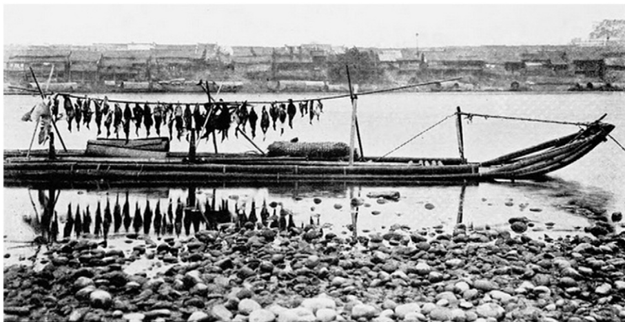
Fig. 2. Heat-bent prow of bamboo boat [4].
