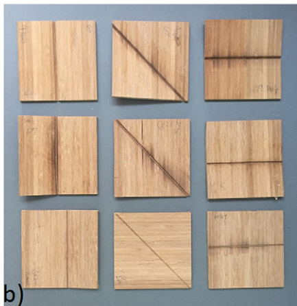
Fig. 11. Scoring and heating tests on depth and orientation to grain on (a) birch plywood and (b) laminated bamboo.
