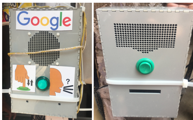
Figure 2: Initial prototypes. Left: the machine-powered-instant system (MPI), showing pictogram signage added after the lab study. Right: the human-powered-delayed system (HPD) in its original form.
