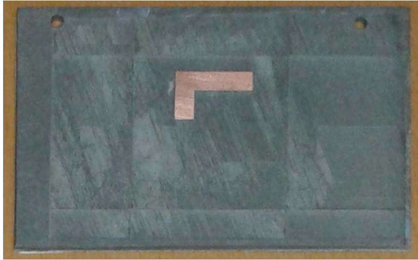
Figure 4. Photograph of the back of the sample: hidden L-shaped metal layer behind a dielectric layer
