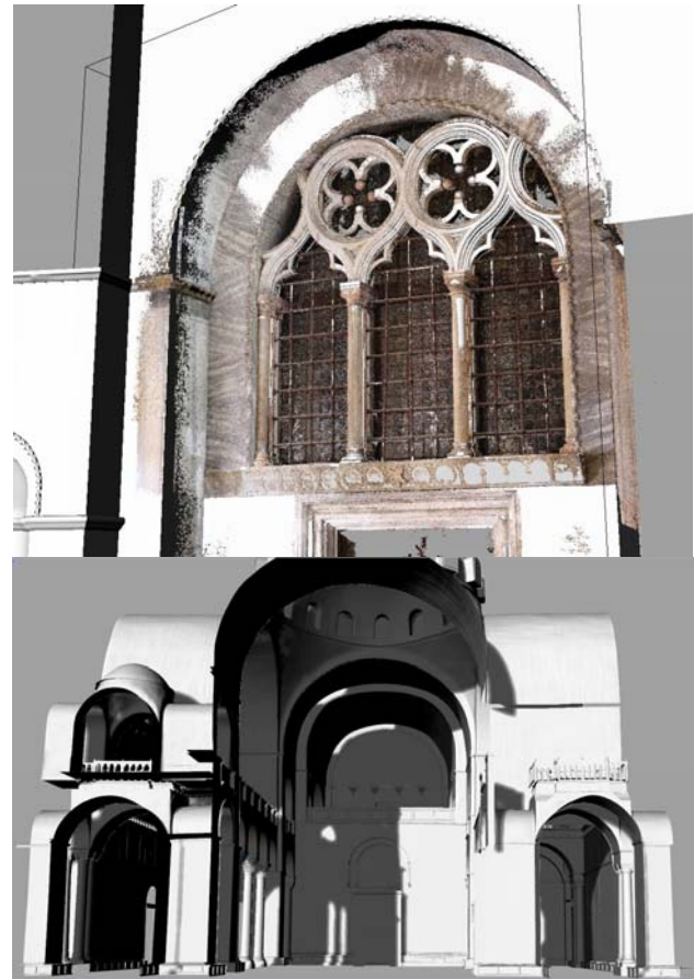
Figure 5: (top) the gothic window of Cappella Zen, is modelled by using sections extracted from the corresponding point cloud. In the image point cloud and NURBS model are overlapped. (bottom) general view of the model
