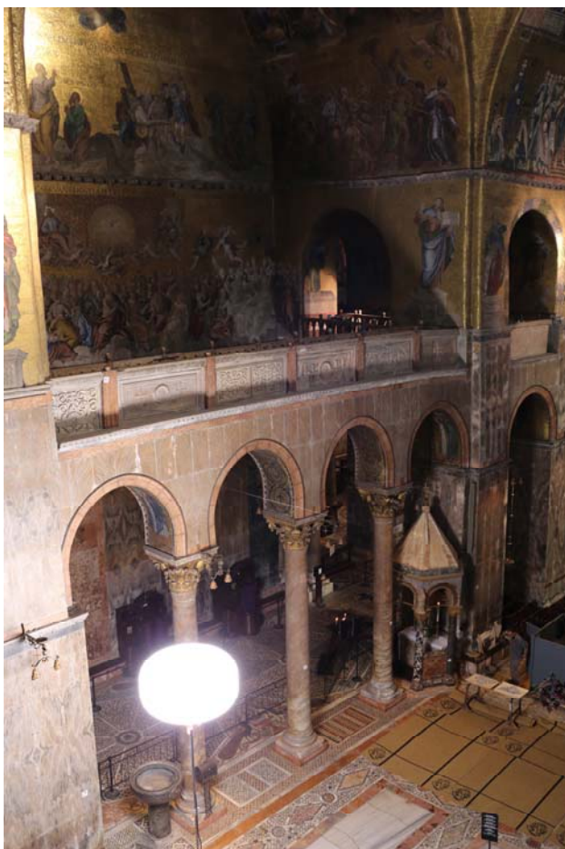
Figure 3: the lighting balloon for the photographic acquisition. It is evident that, even if the balloon is located at a certain height, the higher mosaics are not illuminated.
