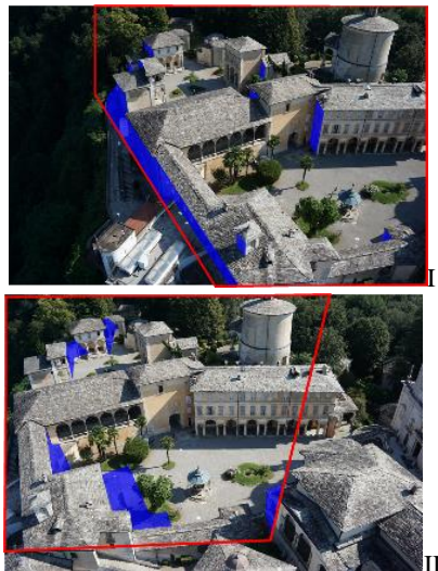
Figure 9. Example of images of two nearest strips in the same flying direction (the same in Figure 8), with underlined an approximated overlapping area (with red borderline) and the respective shadows areas (in blue).
