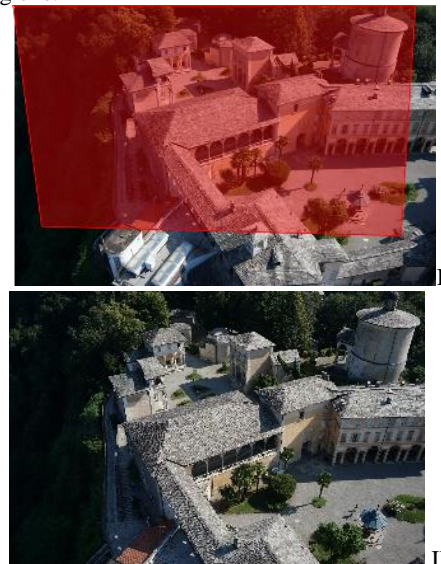
Figure 6. Example of consecutive oblique images with underlined an approximated overlapping area (in red in I).
