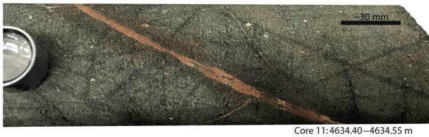
Figure 7. A piece of core from the RN-15/IDDP-2 well from 4634.40 to 4634.55 m depth, showing felsite veins and conjugate sets of older fractures/veins. The red color of the felsite relates to hematic stain formed from a mixture of supercritical vein fluid with cold oxidizing drilling fluid (see text for further discussion).
