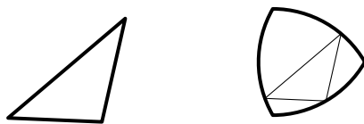
Figure 3.2. Inradius: The set C is a triangle (bold line, left), the set K is a Reuleaux triangle (bold line, right). The inradius r(K, C) is determined by the largest homothetic image of C that is contained in K (thin line).
