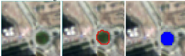
Figure 7. Evaluation. (a) Part of a remote sensing image (b) Output of automatic segment, a roundabout shapefile (c) Manually interpreted roundabout (in blue).
