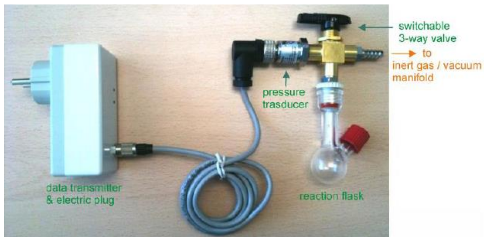
Figure 12. Assembly of the Man on the Moon X102 kinetic kit (obtained from reference 64).
