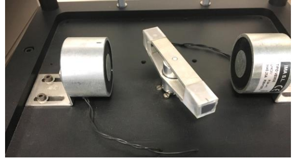
Fig. 9 Structure of the roto-magnet plant
