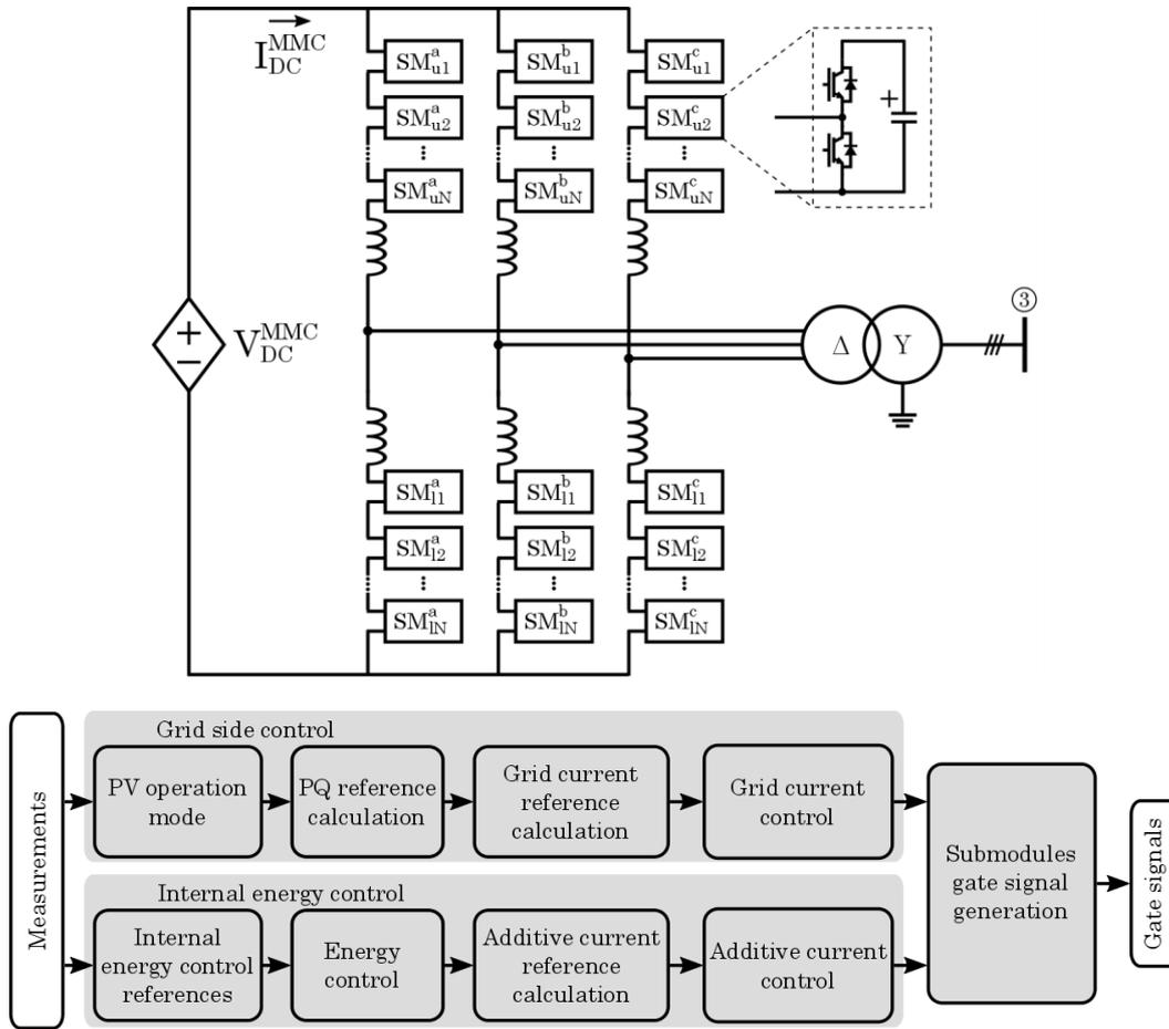
Figure 4. Configuration and control of VSC-MMC-HVDC link
