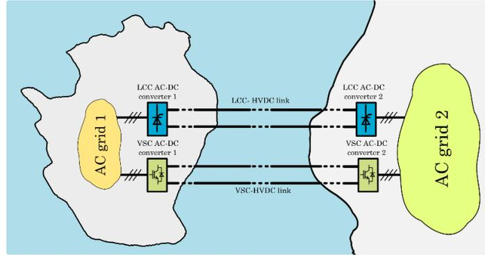
**Figure 1.** Example of dual-infeed HVDC system with LCC and VSC links
