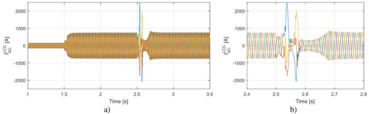
**Figure 7.** LCC AC current during commutation failure
