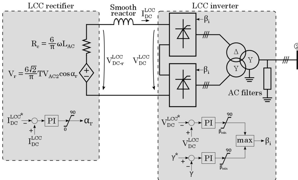
Figure 3. Configuration and control of LCC-HVDC link
