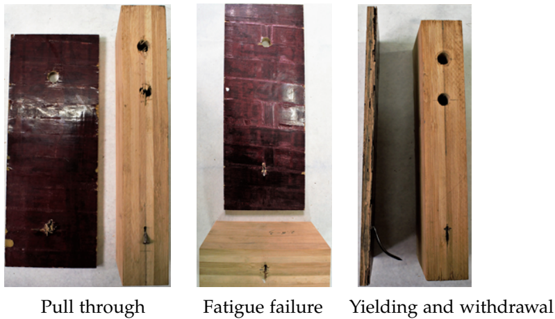
Figure C.5. Failure modes of 60 mm common nails.
