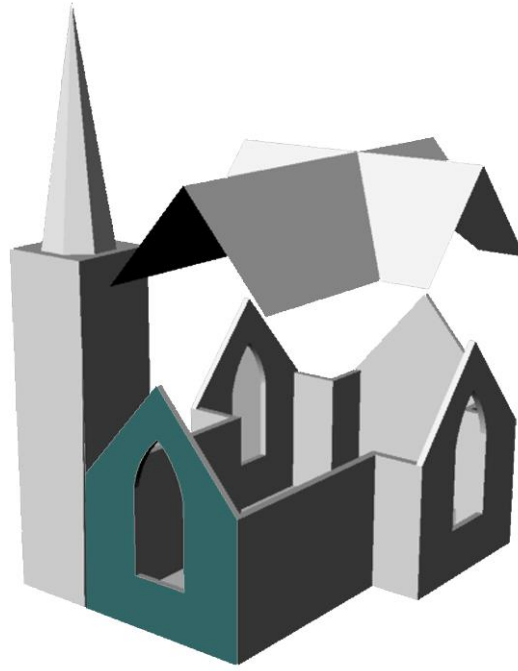
Figure 4.3. Surface area of the façade macroelement (associated to mechanisms #1 and #3) and church total surface area.
