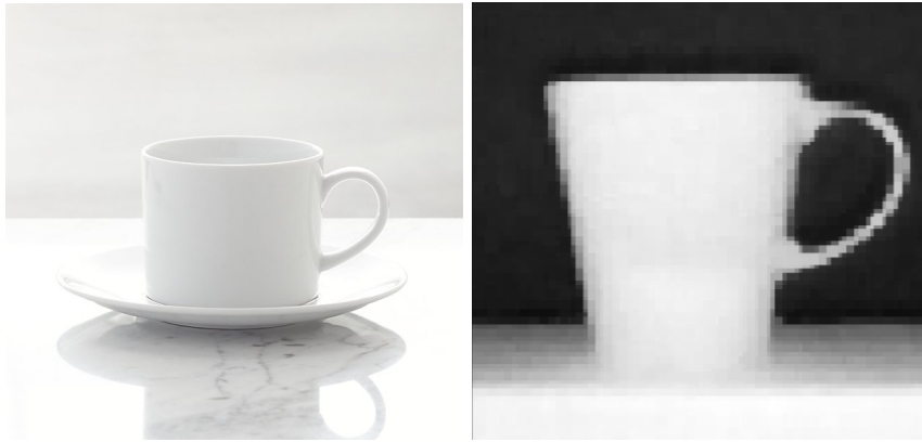
Figure 2.8. To the left: an RGB image of a white cup, on a white plate, sitting on a white table with a white background. Similar scenes lack in texture and are extremely hard to correctly classify. To the right: the depth image of a similar scene. Note how the cup is much more visible against the background and the gradient on the table gives us geometrical intuition.
