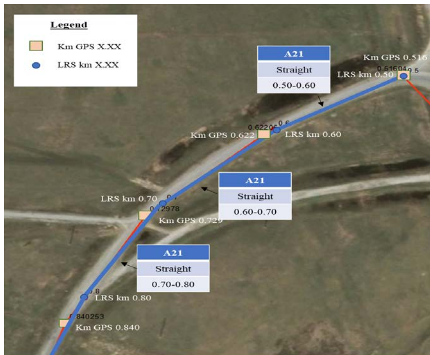
Figure 5-3. Results of the application of GPS matching procedure for the implementation of LRS
