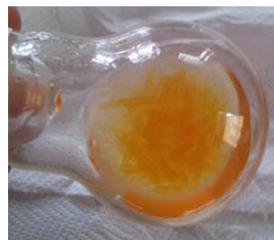
Figure 4.3-8: Photo of tubular structures corresponding to PLL-FA conjugate, achieved using 10% of FA.
