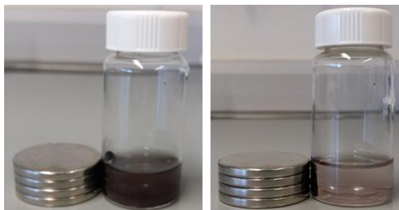
Figure 3.3-3: Magnetic separation of MNPs using external permanent magnets. After few minutes from applying magnets the black solution containing MNPs (left) becomes transparent (right).
