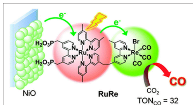
FIGURE 6 | Definition of a photocathode based on nanostructured NiO for the selective photoelectrochemical reduction of \text{CO}_2 to CO. The photocathode is sensitized by a di-nuclear complex of Ru and Re having the dual function of absorbing visible light and transferring electrons to \text{CO}_2 . Reproduced with permission from Takeda and Ishitani (2010).
