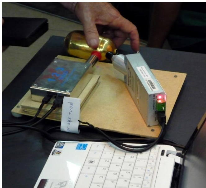
Figure 2. Energy-dispersive X-ray fluorescence portable equipment, composed of a Si-drift detector (on the right; 123 SDD: 450 μm thickness, 7 mm 2 area, and 125 eV energy-resolution at 5.9 keV) and an Ag-anode X-ray tube (40 kV, 100 μA maximum voltage and current) [10]. Electronics including bias supply and Multi-Channel Analyzer (MCA) are in the case of the detector; X-ray tube bias supply is in the case of the X-ray tube. A typical measurement takes 50–100 s.
