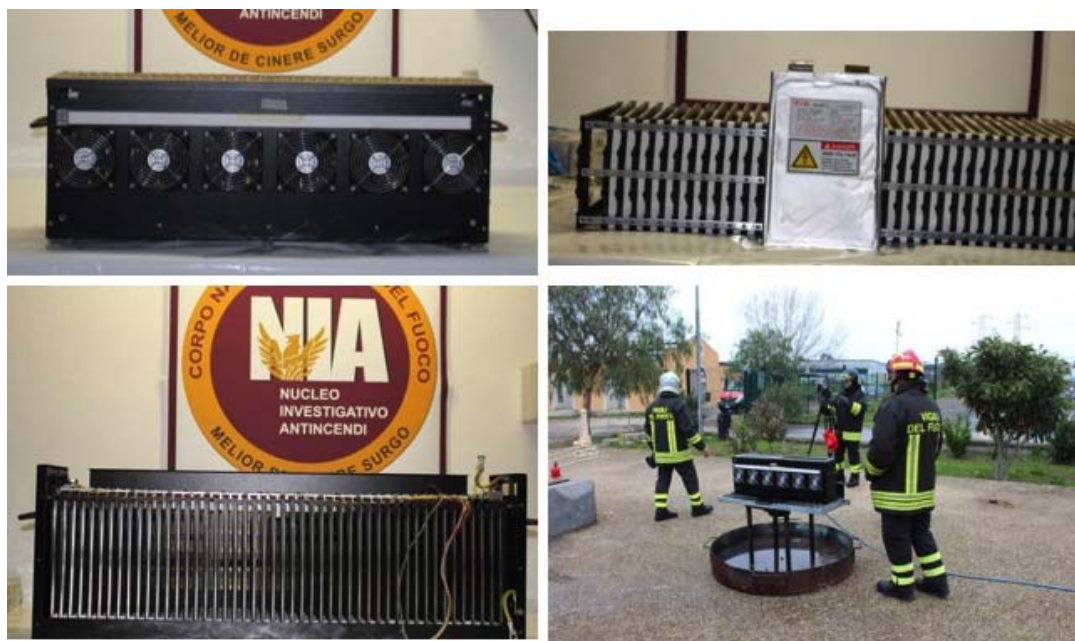
Figure 2 – Battery pack made up of 48 EIG C020 cells.
