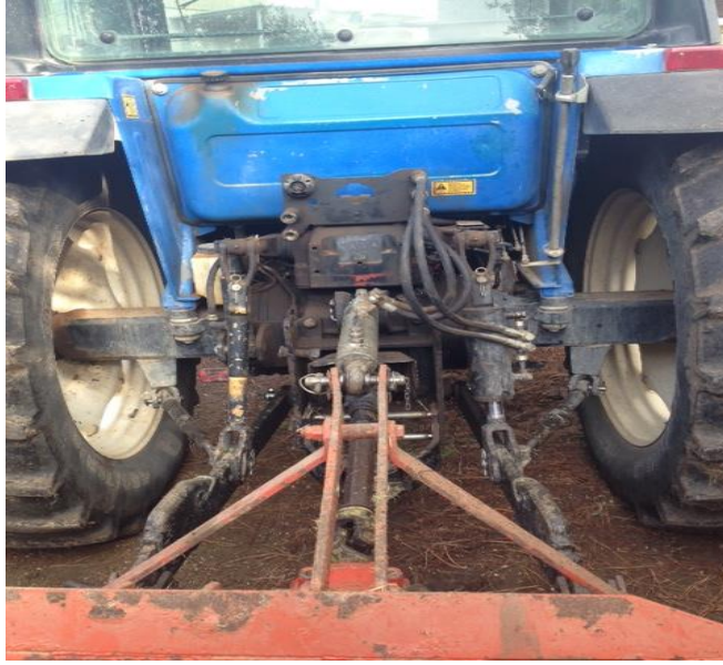
Figure 8. Detail of the tractor's PTO.
