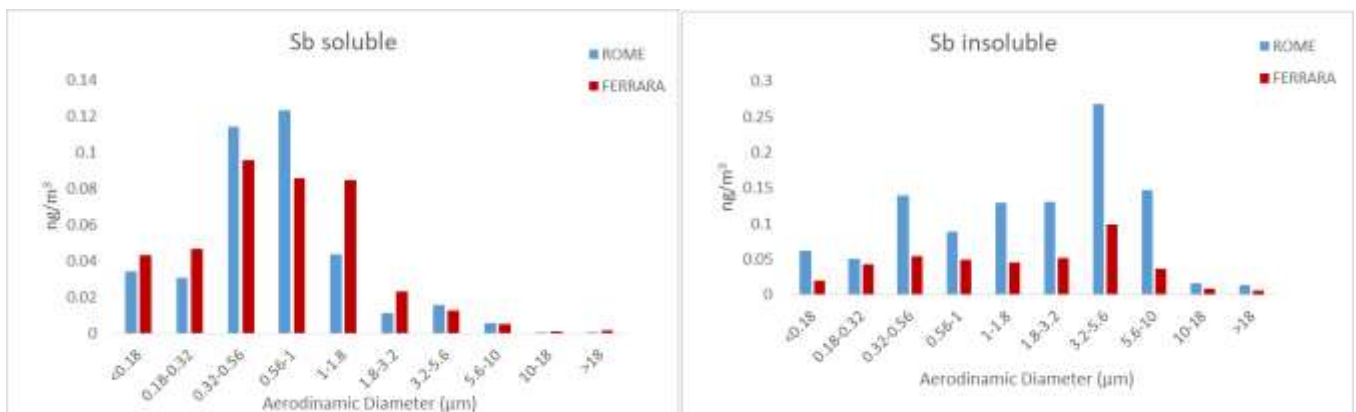
Figure 3: Dimensional profiles of Sb obtained by the analysis of impactor (SOP1 and SOP2)
