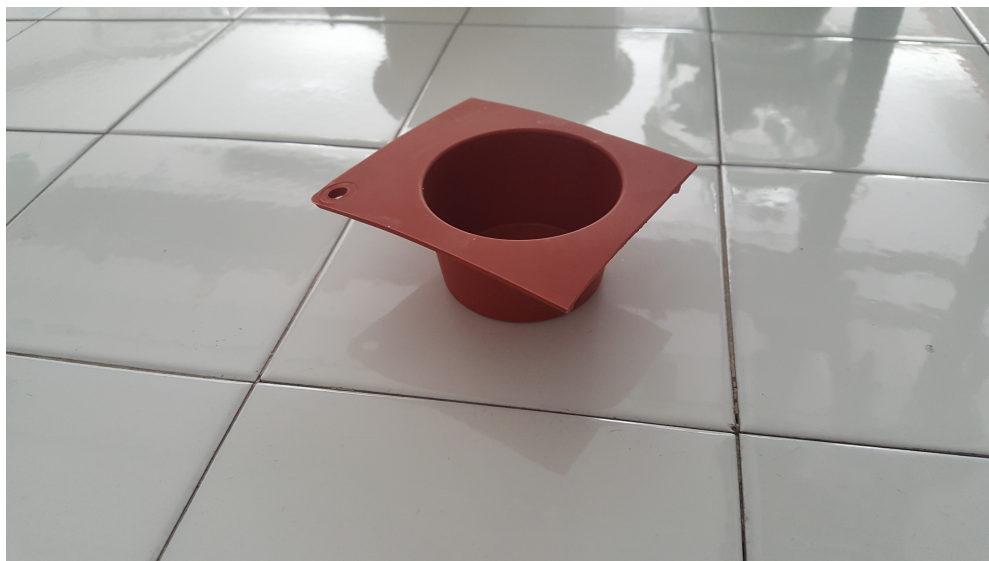
Figure 4.2: Picture of silicon mold for casting solution.
