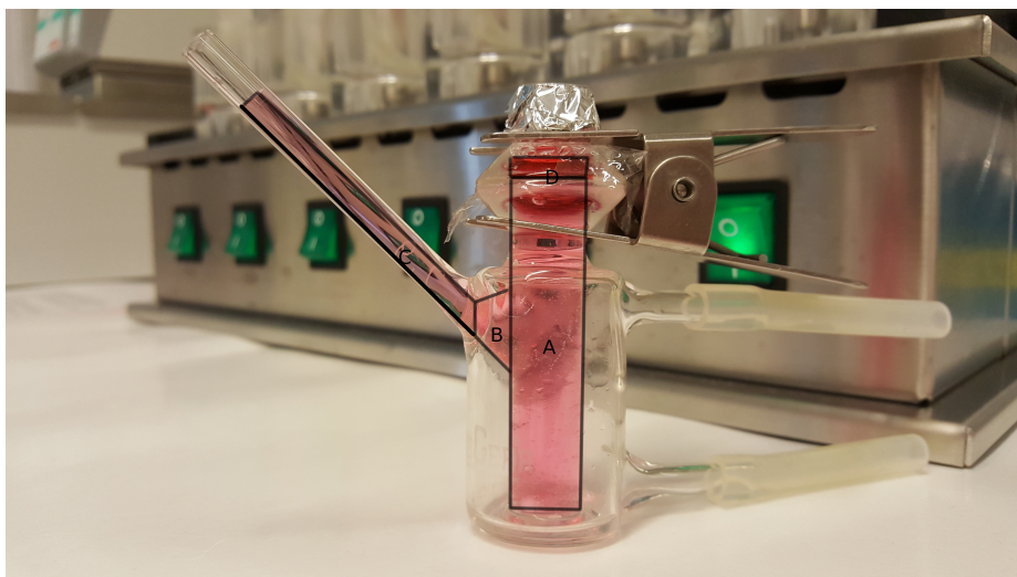
Figure 5.5: Domains within the Franz cell. A) central body, B) connection zone, C) arm, D) membrane.
