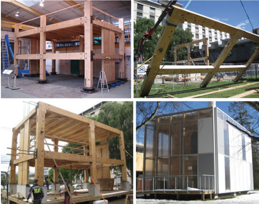
Fig. 13.29 From laboratory specimen to office building: 3D Test Specimen tested in the lab (Newcombe et al. 2010), dismantled and reconstructed (Smith et al. 2011) on UC campus as EXPAN/STIC office
