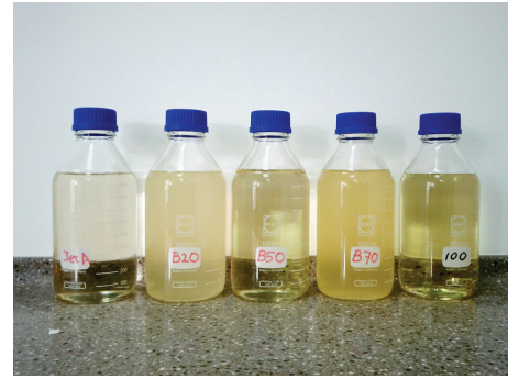
FIGURE 3: Test fuel samples; from left to right: Jet A-1, B20, B50, B70, and B100.
