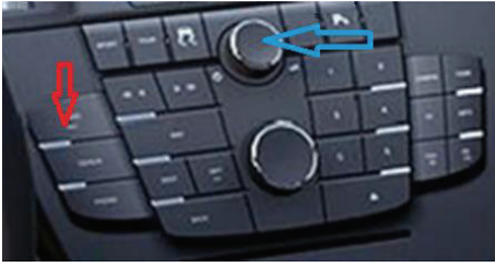
FIGURE 5: The radio used in the radio task. Red arrow points to the correct button for turning the radio on. Blue arrow shows where the participants tried first to start the radio.
