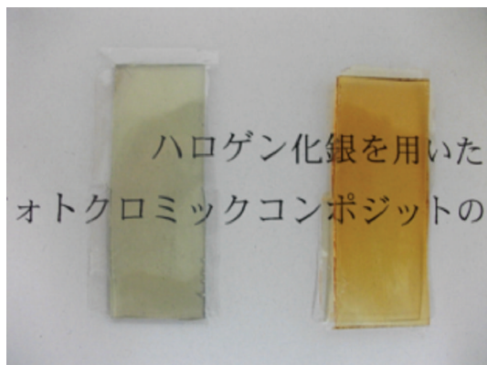
FIGURE 1: Photographs of composite films (Sample 1 in Table 1) before and after UV irradiation.
