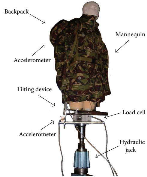
FIGURE 3: The dynamic load carriage test rig. The hydraulic ram drives the mannequin up and down at different frequencies and amplitudes. Accelerometers measure the motion of the backpack and the mannequin, and a load cell measures the dynamic force propelling the mannequin.
