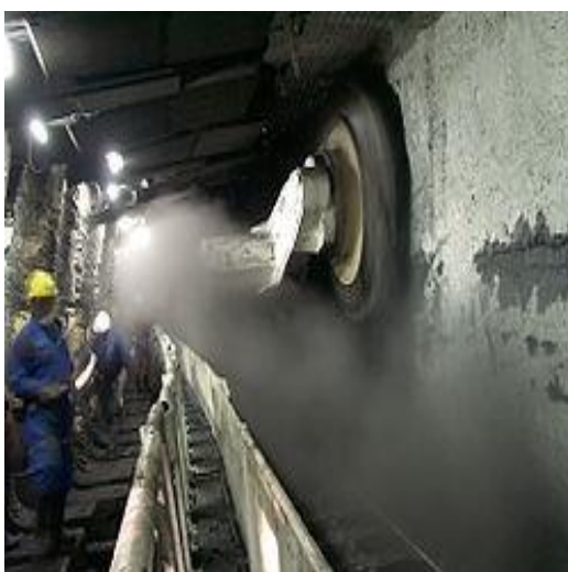
Figure 2.3 Longwall coal face (Chabedi, 2015)
