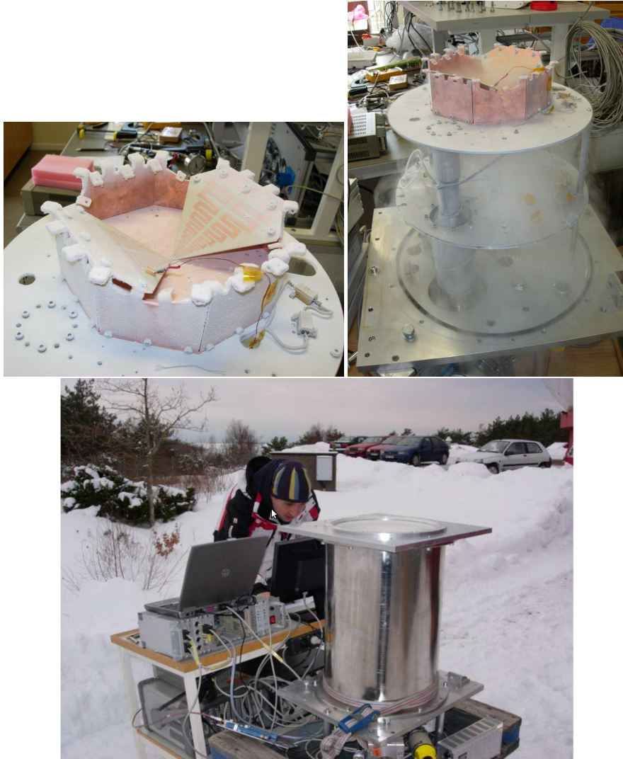
Figure 3.12: Cryogenically cooled Eleven antenna in Dewar, and measurement setup. Liquid Helium is used for the cooling, and the system is given several hours to stabilise. The amplifier voltages were monitored to control for gain fluctuations using a precision power supply.
