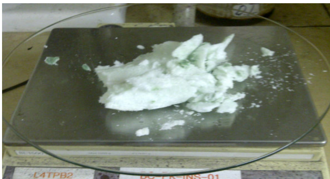
Figure 4-21: Sodium sulphate cake made by controlled agitation from Test 10
