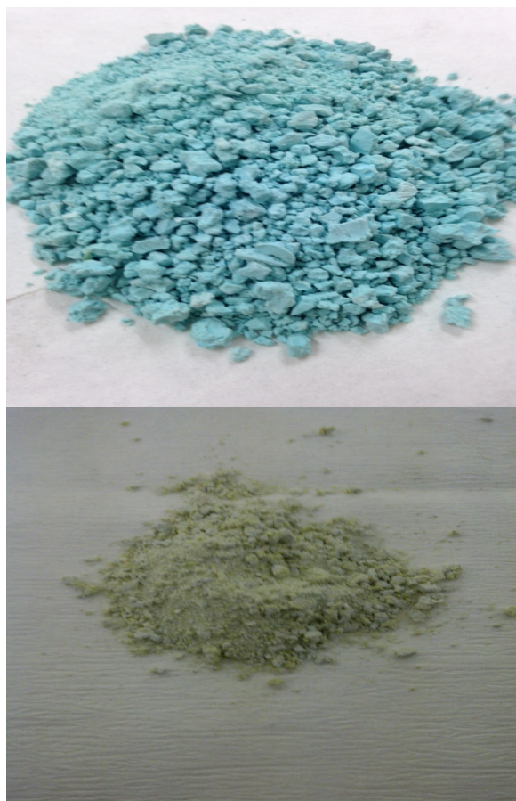
Figure 4-14: Lead-sulphate cake formed from solution with a high copper concentration (left) and cake formed from solution low in copper (right)
