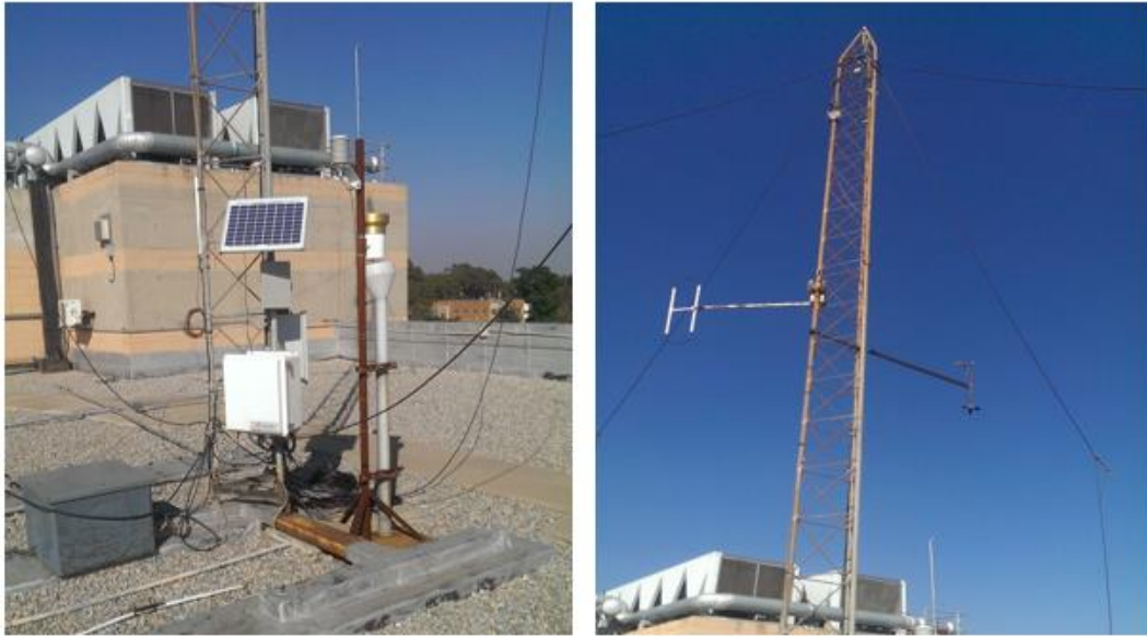
Figure 1- 2 An image of a weather station present at on the surface of the mock underground mine, showing instruments for measuring temperature, humidity, rain water levels and pH (source: Author)
