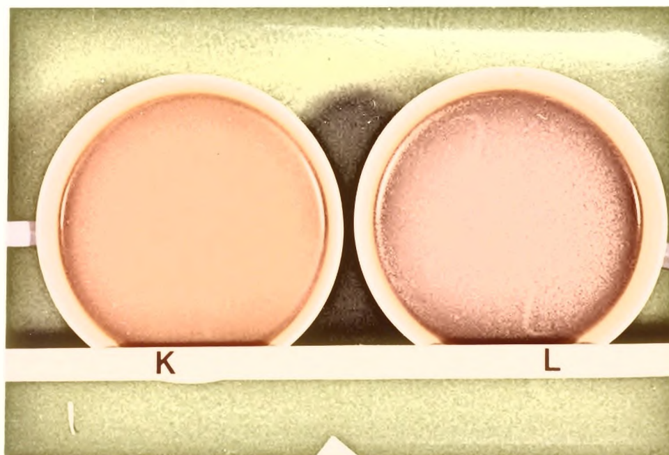
Fig. 23 K White coffee L White coffee + 35.8 \mu mol iron as ferrous sulphate
