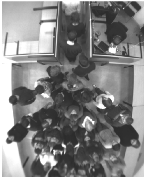
Figure 3.5: The Y or V shape forms around the exit where the clogging occurs
