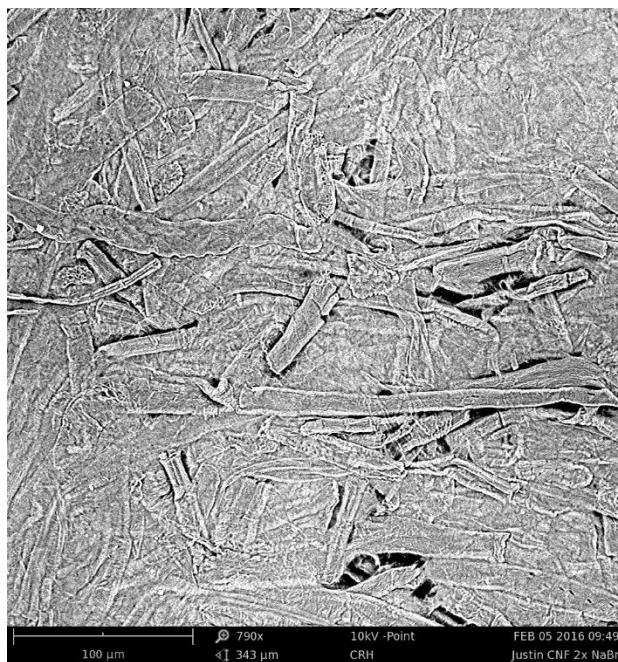
Figure B.28: SEM image of doubled NaBr resolution 790x
