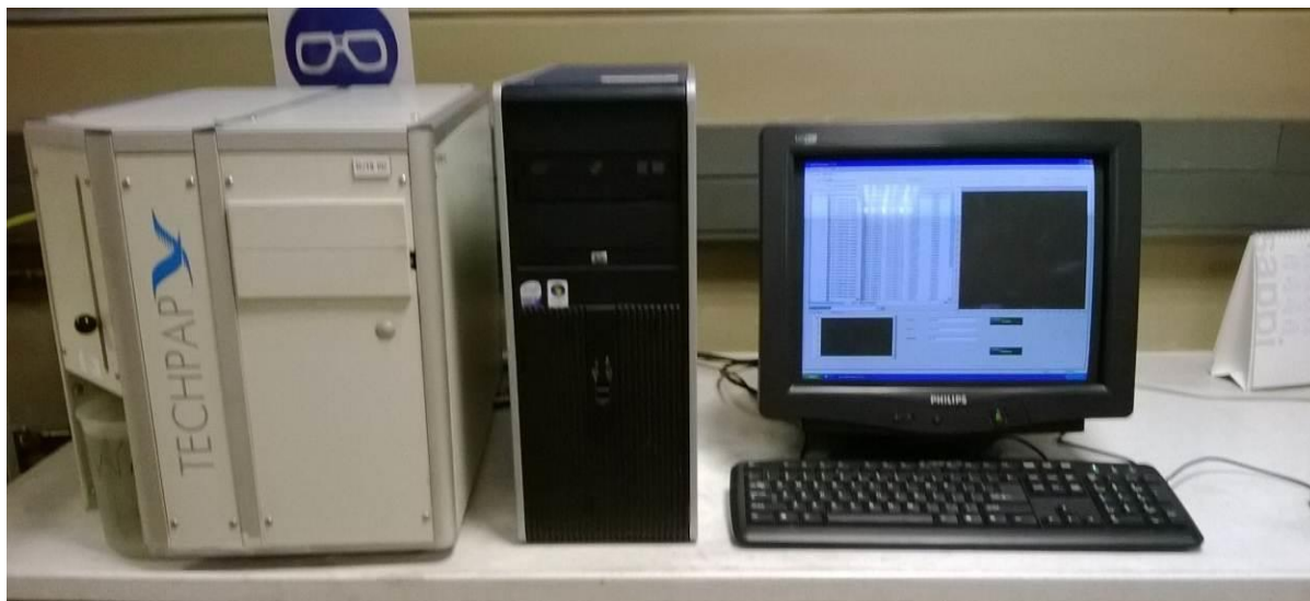
Figure 3.5: TECHPAP Instrument to measure MFWT
