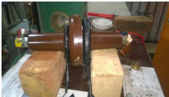
Figure C2: Current impulse tests with type C bushing measured with 418 turns and 875 Rogowski turns coil
