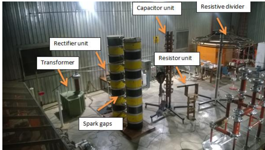
Figure A2: 1.2/50 \mu s impulse generator components
