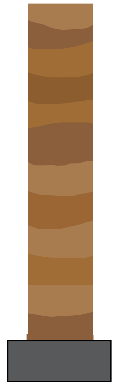
Framework is removed leaving rammed earth wall
