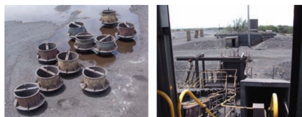
Figure 10—(a) Pots holding up to 1.7 t of ore in which sample material is collected in the metallurgical plant, and (b) railcar loading facility fed by trucks moving material from blended stacks
