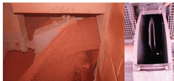
Figure 11—(a) Tippler in motion as 100 t of ore is discharged from a wagon, and (b) cross-belt sampler on iron ore conveyor belt (source: Kumba Iron Ore, 2010)
