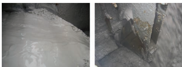
Figure 6—(a) Turbulence created at the 'lip' (LHS of launder) will introduce bias at this point, (b) cutter blades are not long enough to match the flow rate (source: Kelly, 2007)
