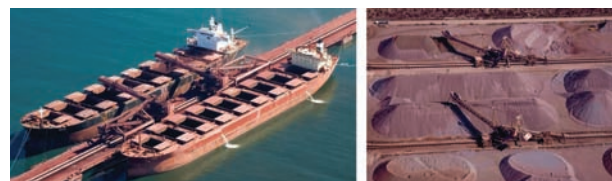
Figure 12—(a) Dual shiploaders at the Saldanha port loading facility, and (b) stacker-reclaimers in the stockpile area at the Saldanha port loading facility (source: Kumba Iron Ore, 2010)
