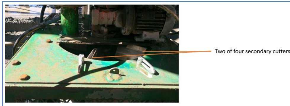
Figure 3.3: Secondary Vezin Sampler with Four Cutter Arrangement.
