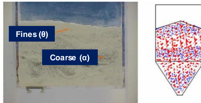
Figure 2.8: Example of Impact Fluidization Segregation. (Johanson, n.d.)
