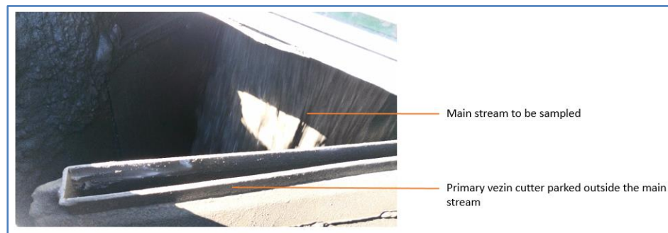
Figure A.2: Primary Vezin Cutter in Stationary Position.
