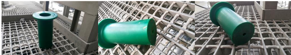
Figure A.10: Old Nozzle Design.
