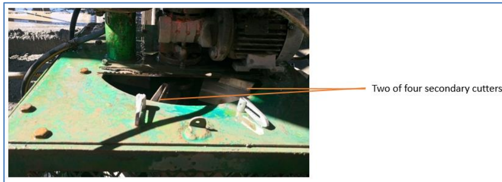
Figure A.6: Secondary Vezin Sampler with Four Cutter Arrangement.
