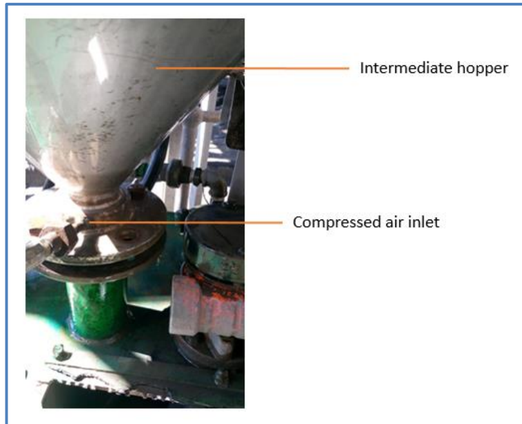
Figure A.4: Intermediate Hopper with Compressed Air Supply Connection.
